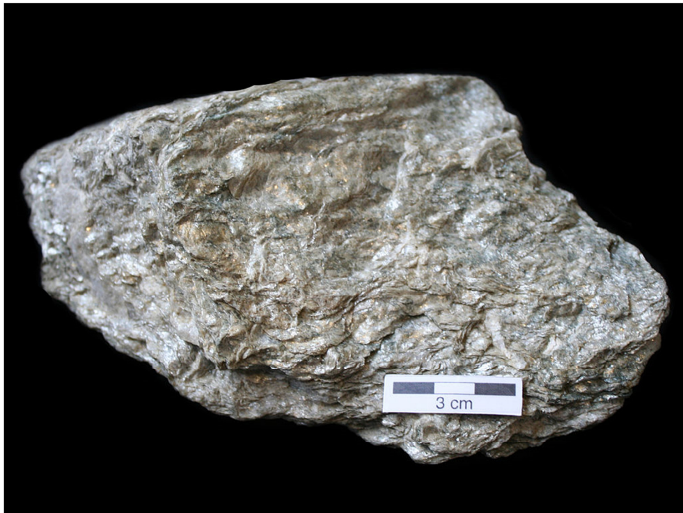
Mica Schist Example. The micas have developed a preferred orientation giving the rock a foliated texture.
