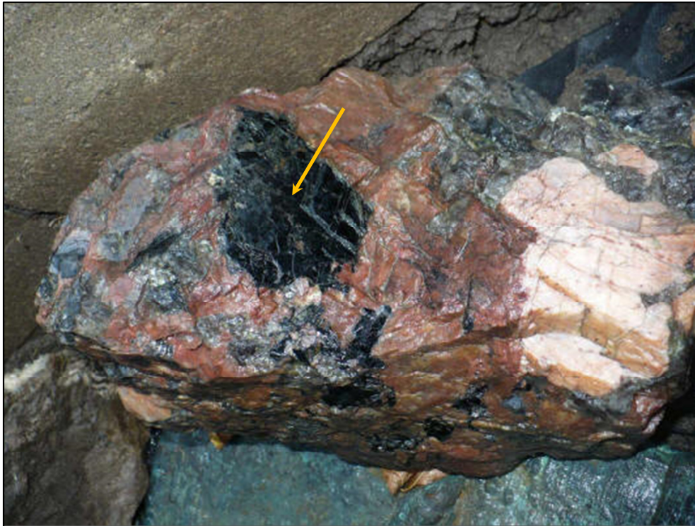
Coarse grained granite specimen with coarse biotite mica (arrowed)
