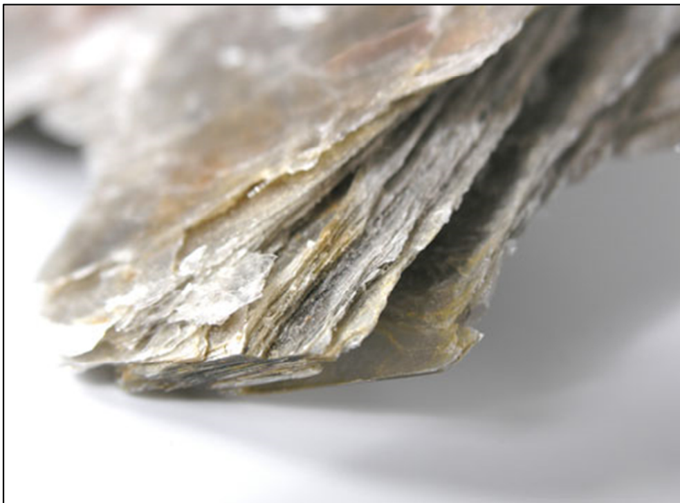
Stacked muscovite crystals showing perfect basal cleavage (planes of weakness)
