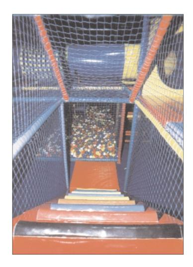
A 5 year old boy was cut across the neck when using a slide during a visit to a pub. An inspection of the play area revealed two loose ropes hanging over the slide, from a piece of netting in which there were holes wide enough to trap a child's limbs or head. The brewery were found quilty of failing to maintain equipment and fined £7,500.
